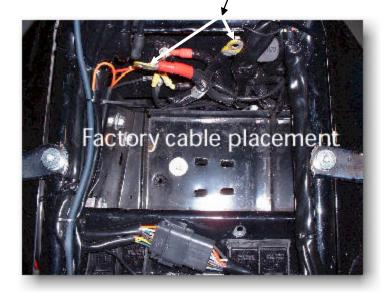
Photo #3 – shows the nut that you will need to loosen so the negative battery cable can be re-routed.
