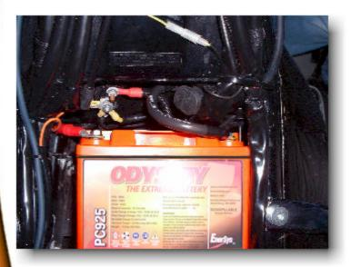
Photo #5 – Install your ODYSSEY battery and attach the cables as shown. The negative cable will clear the seat with room to spare.
